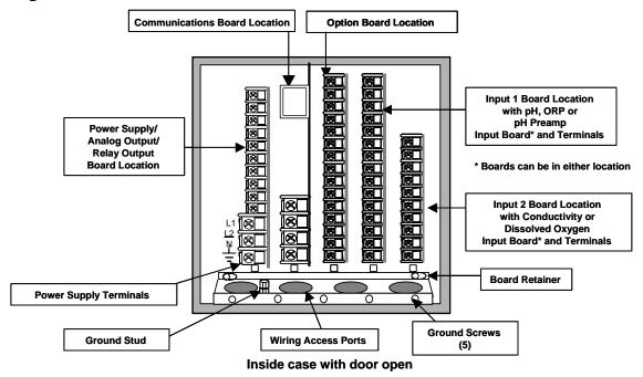
Figure 7-1 Wiring Terminals and board Location
